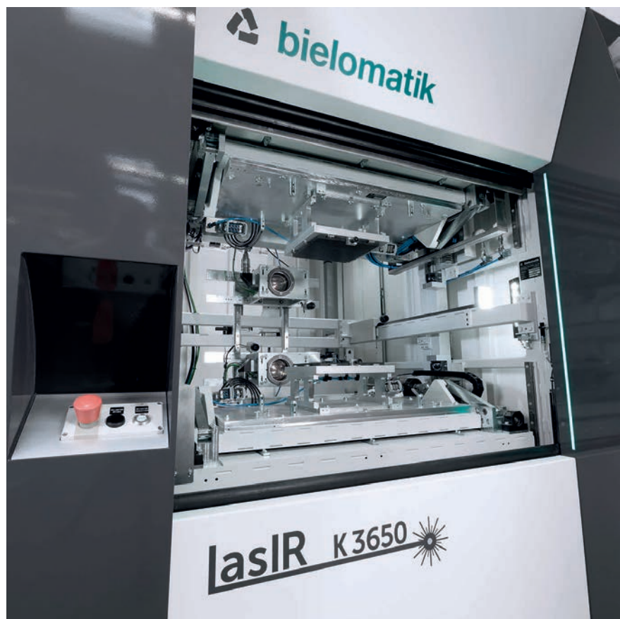
Turn2Weld technique: the newly developed welding machine uses one laser per part and swivels the machine tables through 90° toward the laser scanners with the aid of servo motors (© bielomatik)
