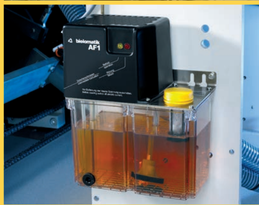
Single line lubrication system within a paper processing system
